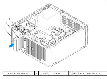
4. Attach the cable to the media card reader and to the system board.
