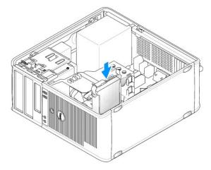
8. Locate an unused SATA connector on the system board and attach a data cable to this connector and to the second hard drive.
