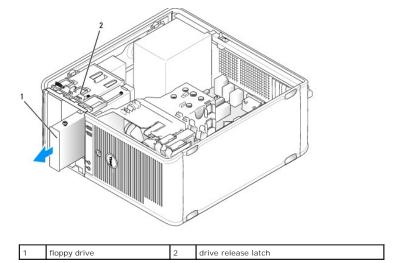
6. Grasp the sliding plate lever and slide it towards the bottom of the computer until the drive panel snaps open; while holding the lever in place, slide the drive out of the computer.
