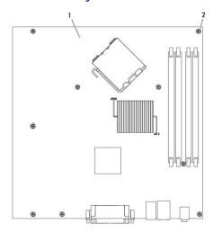
1 mini tower system board 2 screws (9)
