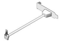
4. Plug the free end of the eSATA cable into the eSATA connector on the system board.
