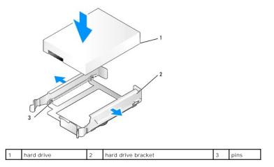
5. Gently spread the sides of the drive bracket and slide the hard drive into the bracket, aligning the drive with the bracket pins, until the drive clicks into place.
