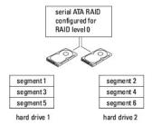
Another advantage of a RAID level 0 configuration is that it utilizes the full storage capacities of the drives. For example, two 120-GB hard drives combine to provide 240 GB of hard drive space on which to store data.
