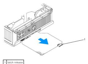
5. Slide the new device into the module bay.
