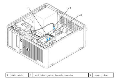
6. Press in on the blue release tabs on each side of the drive and slide the drive up and out of the computer.
